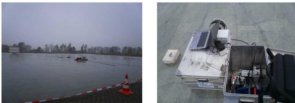
**EXPERIMENTAL SET-UP WITH THE USE OF AN ARTIFICIAL REFLECTOR AT THE ANTENNA REFERENCE OPEN AREA TEST SITE AT PTB (LEFT). DATA WERE CAPTURED AT THREE DIFFERENT ANTENNA LOCATIONS. GEODETIC AND SOFTWARE RECEIVERS WERE USED FOR DATA CAPTURE DURING THE THREE DAYS OBSERVATIONAL PERIOD (RIGHT)**
