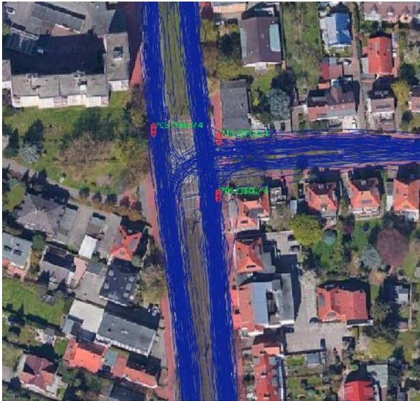
A TRAFFIC LIGHT CONTROLLED JUNCTION SAMPLED FROM DRIVING TRAJECTORIES
