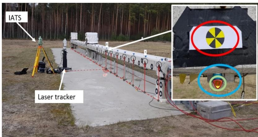
**VIBRATION ANALYSIS OF A SYNTHETIC BRIDGE MEASURED BY THE MEMS ACCELEROMETERS, THE LASER TRACKER AND THE IATS. A PASSIVE TARGET (LOCATED INSIDE THE RED ELLIPSE) ATTACHED TO THE SYNTHETIC BRIDGE, WHICH IS CLOSE TO THE MEMS (LOCATED INSIDE THE CYAN ELLIPSE) AND CORNER CUBE REFLECTOR (LOCATED INSIDE THE GREEN ELLIPSE).**
