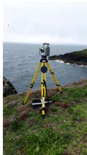
**STATISTISCHES LASER-SCANNING MIT EINER TRIMBLE SX10TOTALSTATION AUF LAMBAY ISLAND**
