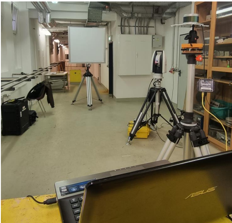
EXAMPLE FOR MEASUREMENT SETUP IN BASEMENT WITH A DISTANCES OF 5 M (LEFT TO RIGHT): REFERENCE PANEL (WHITE, 100%), LASER TRACKER LEICA AT960, VELODYNE PUCK (VLP-16).
